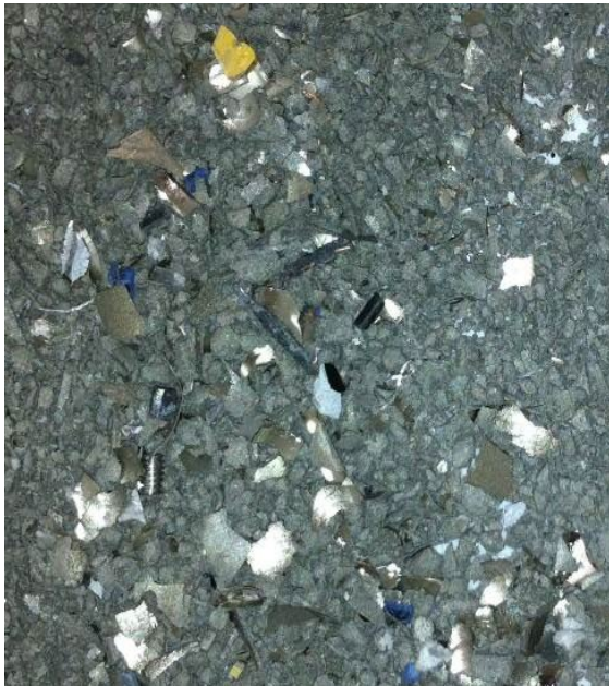
Material extracted from tumbling stage (10 sectioned HDDs).
