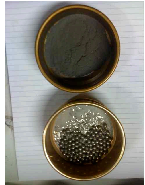
Sieving with ball bearings has been used to preferentially break down the NdFeB compared to the Ni and other impurities
