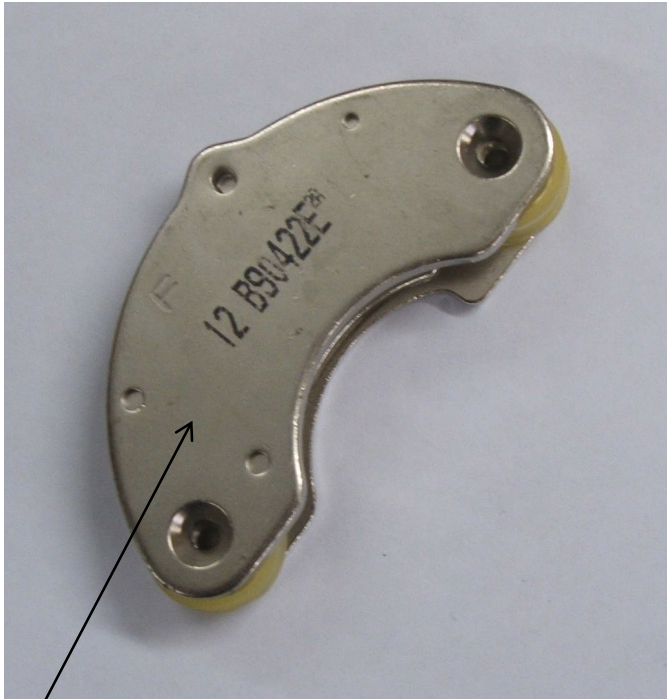
Voice coil assembly extracted from hard drive
