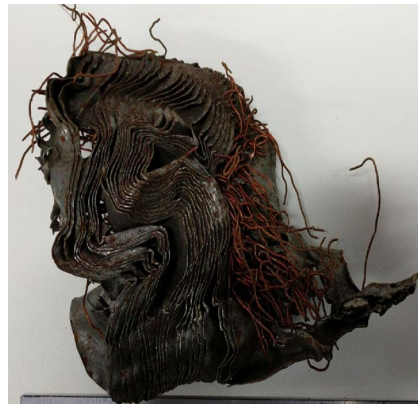
Shredded automotive motor – courtesy of Axion
